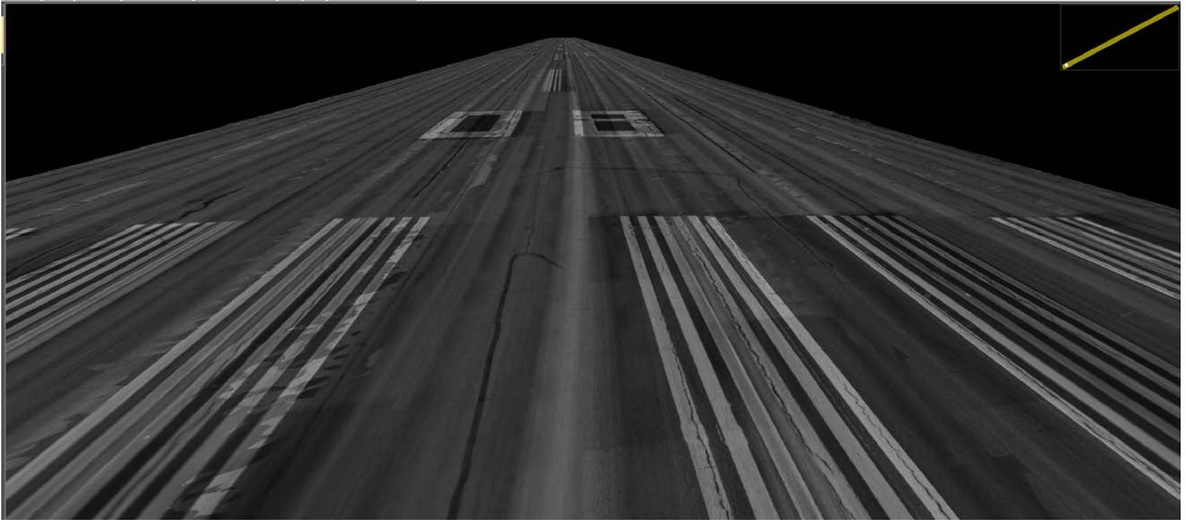
The accuracy of the LDTM solution was evaluated using 44 survey targets which were painted on the runway
