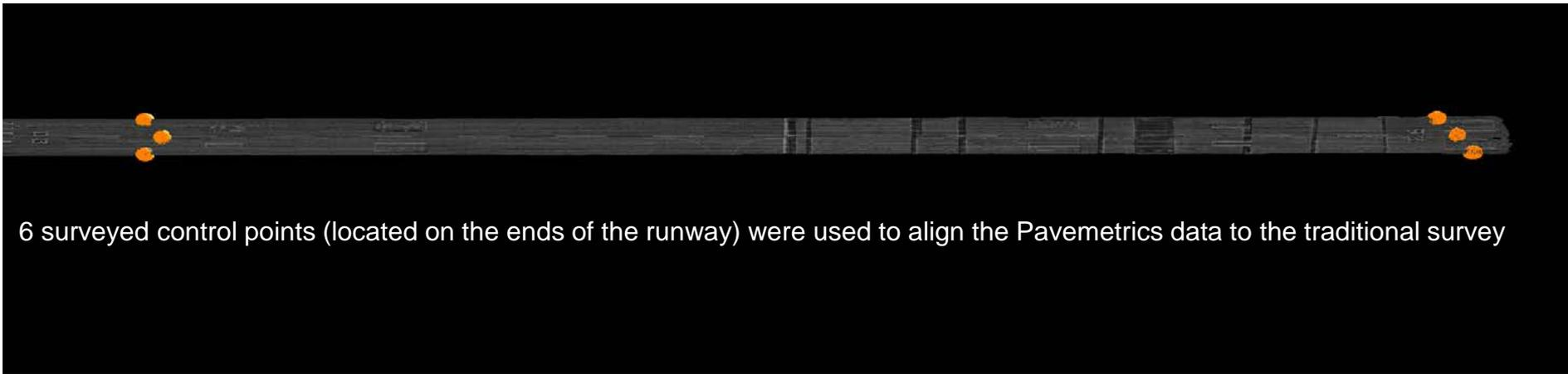
6 surveyed control points (located on the ends of the runway) were used to align the Pavemetrics data to the traditional survey
